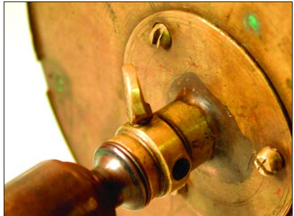
The socket assembly shows the typical diminutive size of the early colonial instruments with the socket plate being made of very thin sheet brass.
