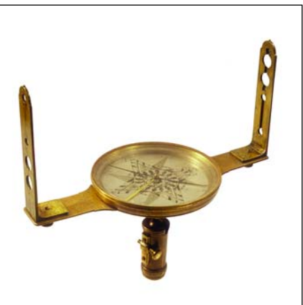
Figure 3 Circumferentor or surveyor's compass
