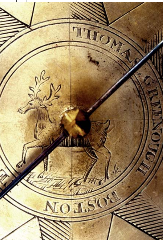
Figure 4 Restored folding sight vane assembly. (As in the case of responsible restoration, all of the replaced pieces on this instrument have been signed and dated so as not to provide any confusing historical data to future research. Under no circumstances should restoration affect the originality of existing pieces of an instrument.) Figure 5 (below) Detailed engraving on a Greenough circumferentor
