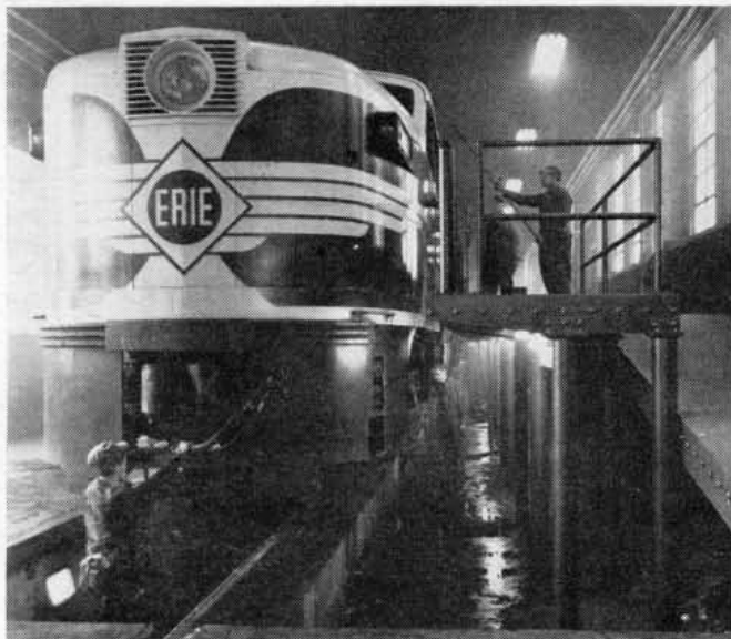
This view shows the three levels on which shopmen can work on a locomotive, the pit, wheel level and door level.
