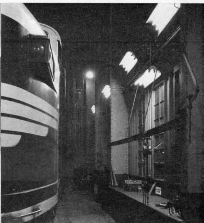
Note the brightly lighted, convenient work bench at right with its own handy crane for quick jobs.
