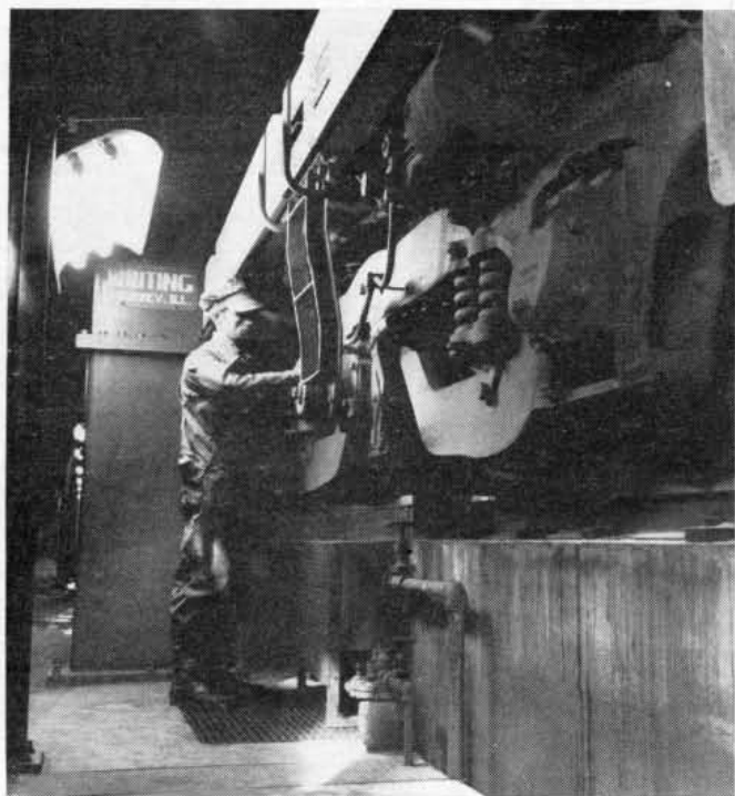
Excellent lighting enables this workman to clean and adjust wheels and truck under safe, bright recessed lights.
