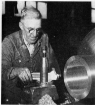
A real veteran, JAMES NEARY, machinist, checks a diesel engine part which he is machining on a lathe. He has been with the Erie 52 years and knows his job so well he can estimate machined parts to a thousandth of an inch.
