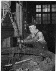
WILLIAM ANISKIEWICZ, machinist, uses a wrench as he works on a traction motor in the Jersey City diesel shop.
