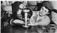
ALFRED DOENO, machinist, operates an instrument for testing various gauges used on locomotives and in the shops.
