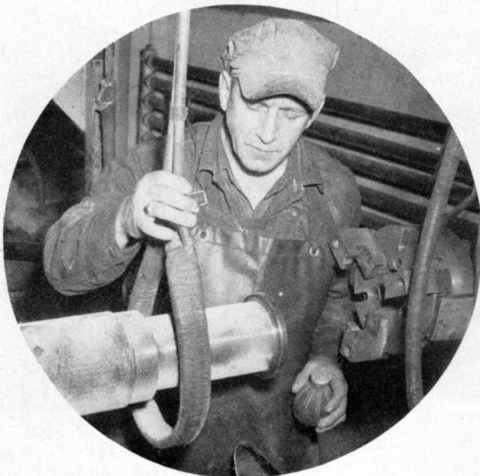
Paul Seaman, machinist, testing car axles before they are fitted with wheels
